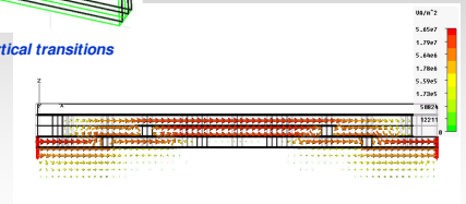
Cross section of the CPW to SL vertical transition
